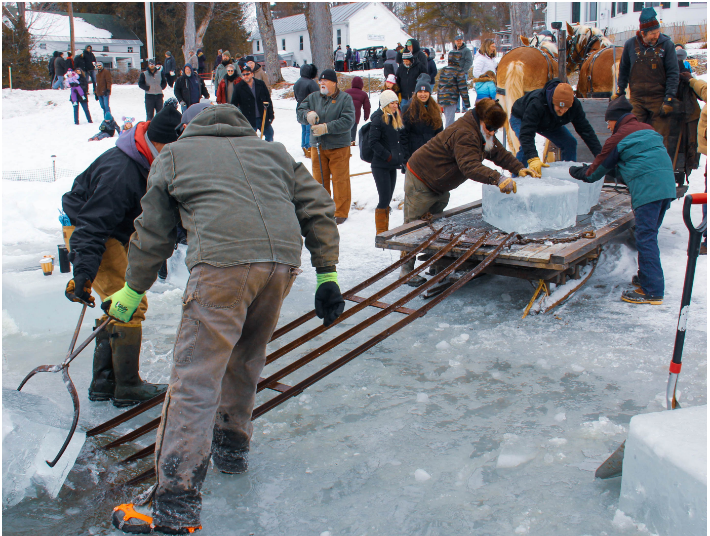
Using tongs to drag the ice blocks onto a horse drawn sleigh for transportation to the ice house for storage.
