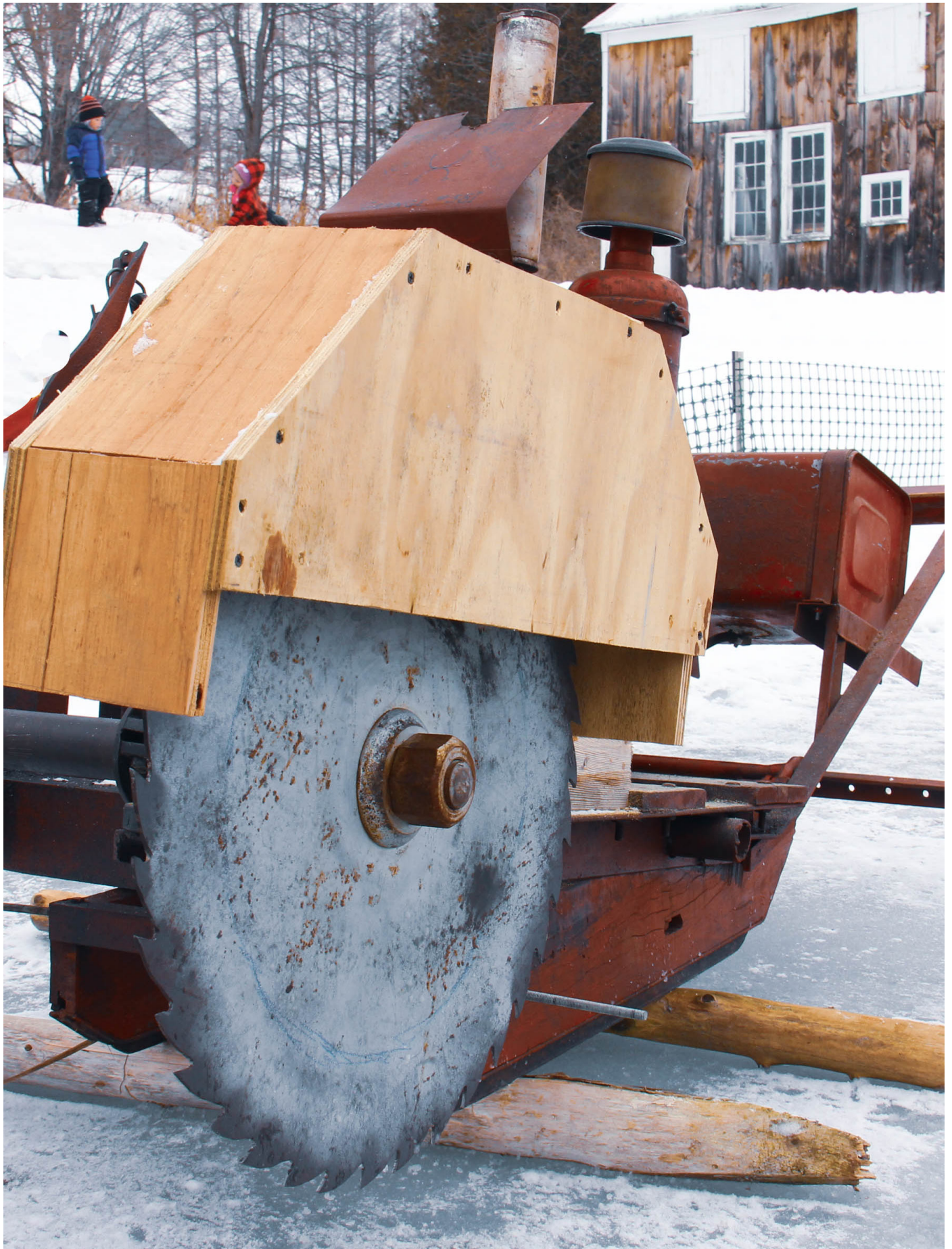
The cutting blade used to "score" the ice for the saws to cut along.
