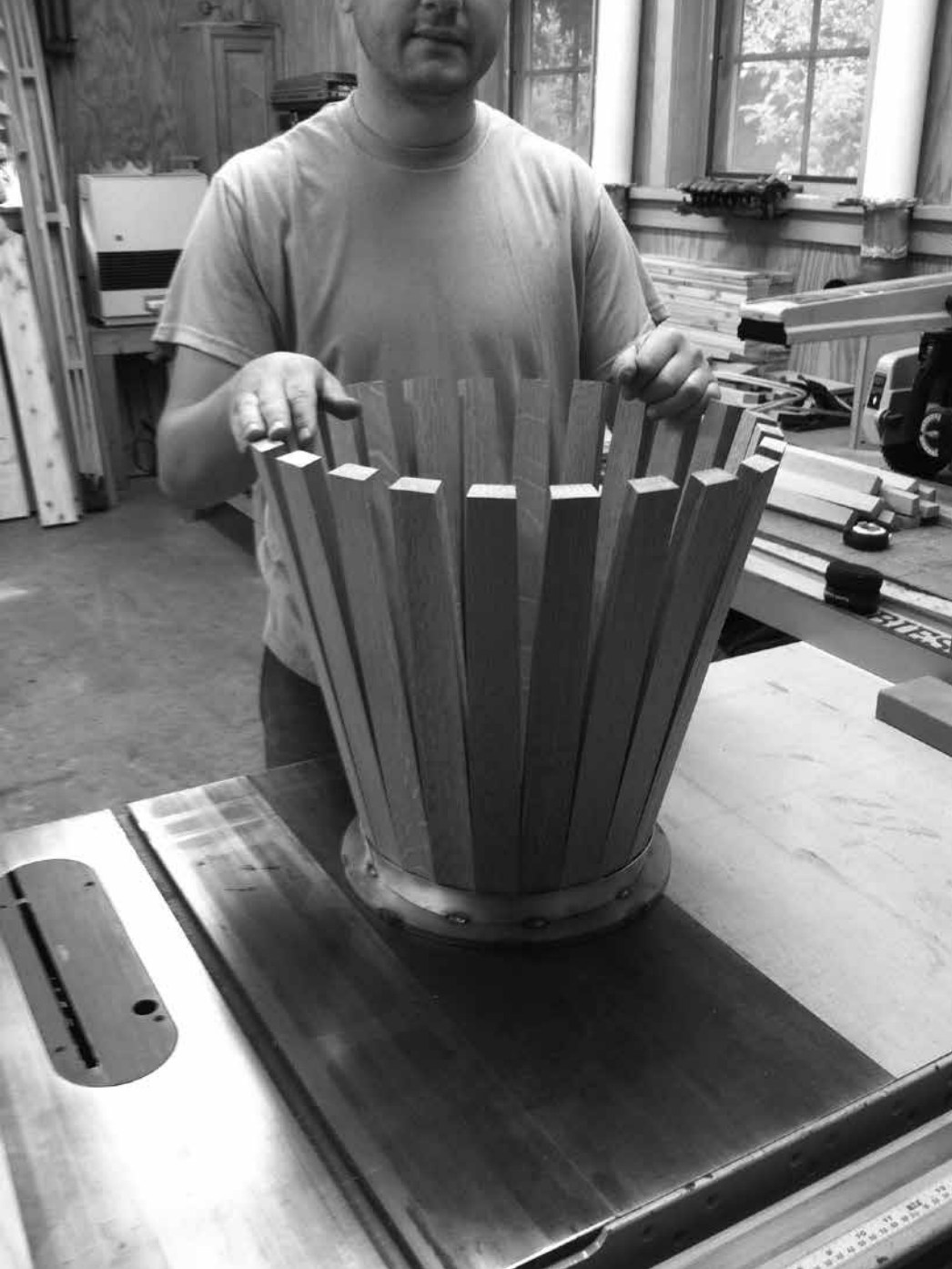
Bob Hockett's employee, Justin Bidelspach, with the first of the two 5-gallon, all-New York oak barrels during coopering. This stage is known as "raising" the barrel, wherein the staves are set on end, bound in place and ready for steaming.
