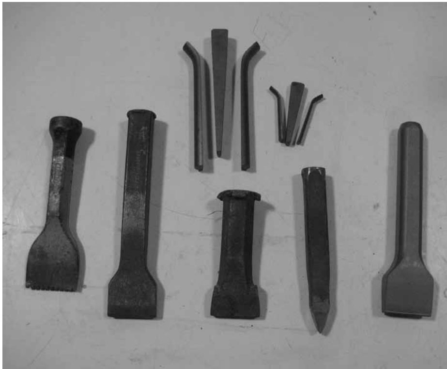
Tools of the trade, including pitching tools, pin and feathers, and dressing chisels.
