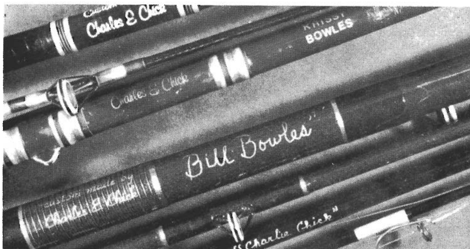
Colored threads are used to hold fishing line eyelets on fishing rods designed by Charlie Chick, Albion, Orleans County. Charlie makes specialized fishing rods for stream and creek fly casting and deep lake salmon fishing. (Photo by Dr. James Orr)
